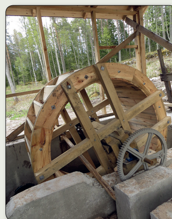
The new waterwheel, reconstructed from preserved parts and a photograph from the 1950s. Photo: Jönköping County Museum.
